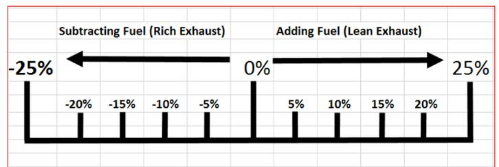
If one bank reading rich or lean, than any concerns that are common to both banks can be ruled out, such as faulty MAF sensors, fuel delivery system concerns, fuel concerns, EGR and air intake system concerns such as vacuum leaks. Items that should be looked at would be specific to that bank, such as individual injectors, vacuum leak on one bank, plugs and/or coils.
