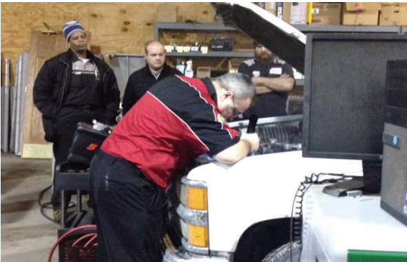
As seminar attendees look on, Ken Dotzler demonstrates various smoke machines to diagnose evaporative emission failures.
