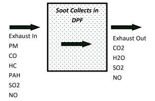
DPF is a honeycomb structure that exhaust must pass through to collect particulates (soot). The DPF is capable of removing more than 90% of particulate matter from the exhaust.
